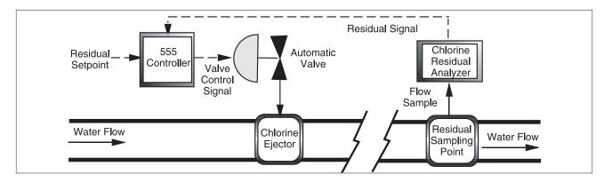
Residual control positions a chlorine valve based on chlorine residual measurement. With a user-defined residual setpoint, the 555 increases or decreases the gas feed rate dependent on deviation from setpoint. Ease of use is provided by continuous readout of chlorine residual and setpoint. Improved residual control is made possible by a fixed lag time function incorporated in the 555. Controllers without a lag time function have to be tuned for very sluggish
