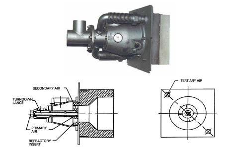
The 1440 Burner Series combines Bloom's renowned low NOx baffle with air staging. NOx levels previously unachievable without exhaust gas recirculation have been accomplished with this breakthrough design.
