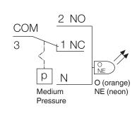
**GMH (Operating state shown) As pressure rises**, 2 NO closes, 1 NC opens, and Neon light ON (fault), switch trips and locks out.
