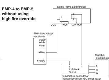
Typical Flame Safety Inputs EMP-4 to EMP-5 using high fire override COM Hig Low Rur EMP-5 is not a di-EMP-5 low voltage rect replacement in input leads this case. Additional Violet/ White wires detailed here Violet are needed. Wire nut -Blue 135 Ohm Potentiometer +Yellow 4 - 20 mA Output Temperature controller or
