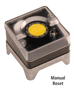
The Versa Plus gas pressure switch accurately monitors pressure and breaks the electrical control when pressure rises above or drops below the desired setpoint. It is made with a durable plastic enclosure and has a die-cast aluminum inlet base.
