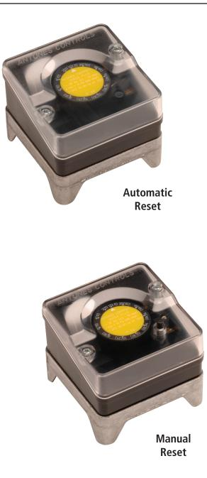
The Versa Plus gas pressure switch accurately monitors pressure and breaks the electrical control when pressure rises above or drops below the desired setpoint. It is made with a durable plastic enclosure and has a die-cast aluminum inlet base.
