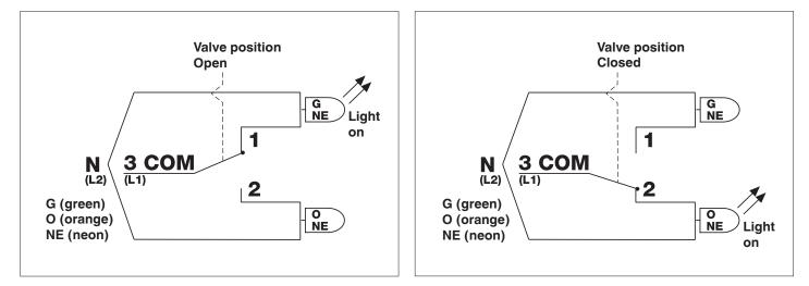
Visual Indicator indicates closed and open position of the safety valve
