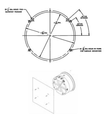
Locate 4 mounting holes, 35° from horizontal centerline on a 4-11/32" dia. circle. Use No. 6-32 machine screws of appropriate length. Be sure to drill 1/4" holes for blowout protection as shown in the diagram.
