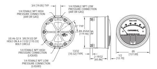
**CAUTION:** Use of a line filter (Dwyer Instruments, Inc. model A-391 or equivalent) is recommended to prevent entry of liquid borne particles into gage. Dwyer Instruments, Inc. cannot assume responsibility for failure of gages due to clogging of internal passages.
