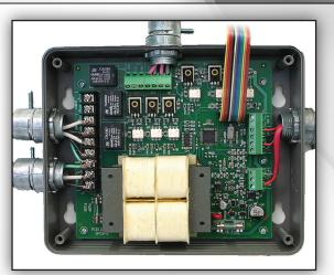
"Under the cover", the Smart System MTLC utilizes a microprocessor based control board to control up to 3 different hydronic heating loop temperatures while maximizing the boiler system efficiency.
