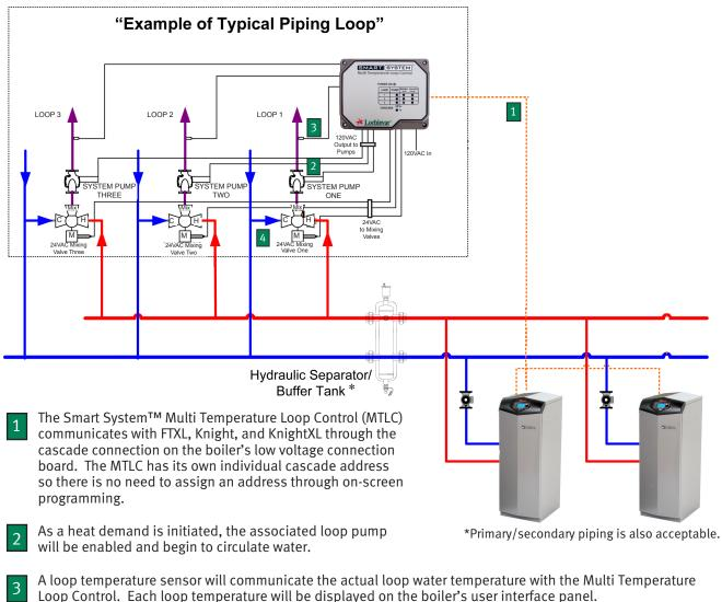
4 The MTLC will actuate the three way valve via a 24 VAC signal to meet the required setpoint. As space heating water temperature approaches setpoint, the MTLC will actuate the three way valve to keep the loop temperature within the programmed range. Indicator lights on the MTLC will display cascade communication with the boiler, pump status and three way valve activity.
