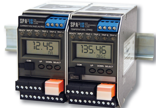
The SPA 2 IS features a metal, RFI resistant housing with display that snaps onto standard DIN-style rails.
