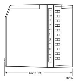
Fig. 1. Mounting dimensions of S7830 Expanded Annunciator and Q7800A Wiring Subbase in in. (mm).
