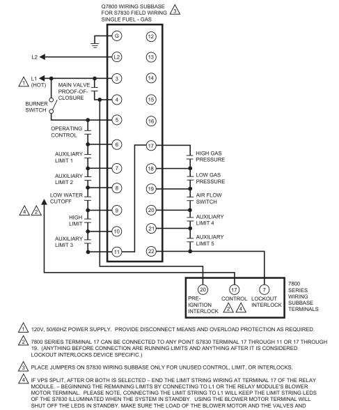
Fig. 4. S7830 wiring hookup—Valve Proving devices with Valve Proving enabled.
