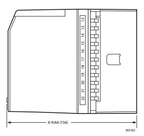
Fig. 2. Mounting dimensions of S7830 Expanded Annunciator and Q7800B Wiring Subbase in in. (mm).
