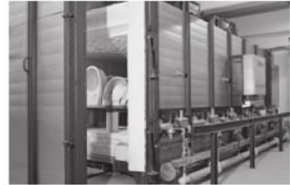
Intermittent shuttle kiln in the ceramics industry
