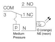
**GMH** (Operating state shown) As pressure rises, 2 NO closes, 1 NC opens, and Neon light ON (fault), switch trips and locks out.
