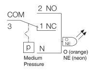
GML (Operating state shown) As pressure falls, 2 NO opens, 1 NC closes, Neon light ON (fault), switch trips and locks out.
