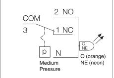
**GML** (Operating state shown) As pressure falls, 2 NO opens, 1 NC closes, Neon light ON (fault), switch trips and locks out.
