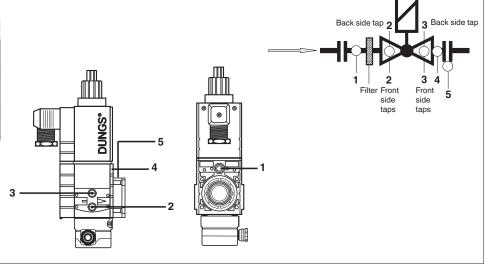
Gas Pressure Switch for DMV safety shutoff valves
