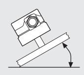
When installed in other position the pressure switch switches at pressure deviating from the set reference value by max.  $\pm 0.2$  in. W.C. (0.5 mbar).
