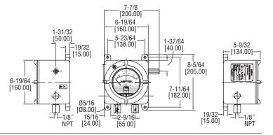
The popular SERIES AT22000 Magnehelic® Differential Pressure Gage is now available in a flame-proof ATEX enclosure with the new ATEX approved AT22000 Series. This gage can indicate positive, negative or differential pressures and is accurate within 2%.
