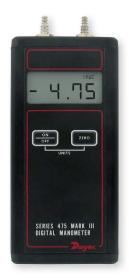
The Series 475 Intrinsically Safe Handheld Digital Manometer measures positive, negative, or differential pressures of air and natural gases in ranges from 1 in w.c. (0.249 kPa) to 150 psid (10.34 bar). The dual push pads on the front panel control the on/off, auto zero, and pressure unit selection, allowing for simple operation with no set up needed. When used with a Dwyer<sup>®</sup> Pitot tube (●), the Series 475 can also be used as an air velocity gage.
