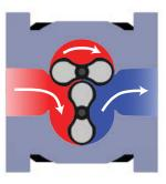
After further rotation the top impeller becomes horizontal and a finite volume of gas is captured in the top cavity.
