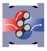
As the impellers continue to turn, the volume of gas in the lower cavity is discharged. Simultaneously, gas is entering the space between the top impeller and housing.
