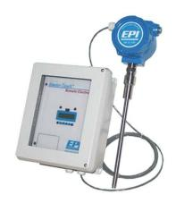
rating and is usually placed in a readily accessible non-hazardous area (Ordinary location). Optionally available, is an Explosion-proof remote enclosure. The enclosure contains the electrical connections, signal processing electronics and the LCD display, with programming keypad. Only a four-wire, twisted-pair cable is required to carry the input power and flow signal between the two enclosures.
