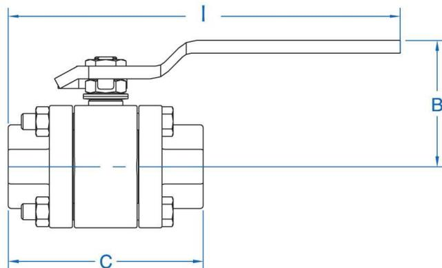
Serie 400 (Latón) Paso reducido • Series 400 (Brass) Reduced bore
