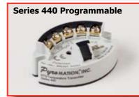
The Series 440 programmable RTD temperature transmitter is a two-wire transmitter with an analog output. It has measurement input for Pt100 resistance thermometers (RTD) in 2 or 3 wire connection. Setting up of the transmitter is done using the 440-CABLE. These small units can be mounted in Pyromation heads or they can be used for surface mounting by using a 35 mm DIN rail mounting clip.
