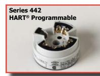
The Series 442 programmable HART® temperature transmitter is a two-wire transmitter with an analog output. It has measurement input for resistance thermometers (RTD) in 2, 3, or 4 wire connection, thermocouples, resistance and voltage. Setting up of the transmitter is done using the 442-MODEM or HART® handheld communicator (275/375). These small units can be mounted in Pyromation DIN (Form B) heads or they can be used for surface mounting by using a 35 mm DIN rail mounting clip.
