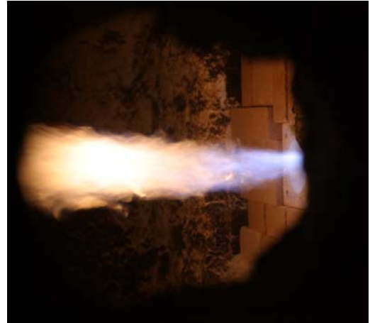
OXY-THERM® LE staged flame pattern
