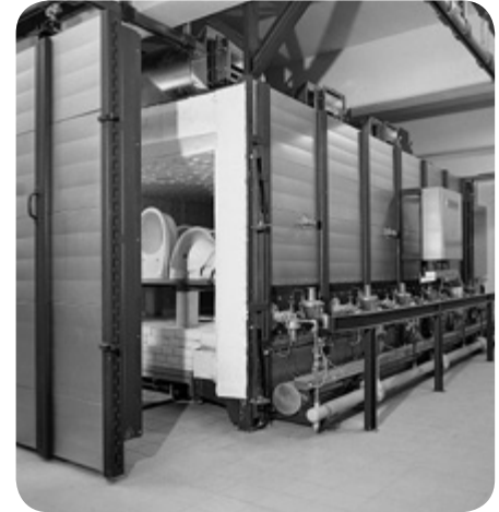
Intermittent shuttle kiln in the ceramics industry
