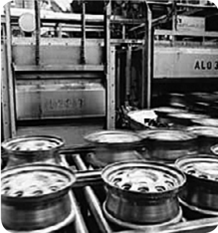
Wheel rim hardening installation
