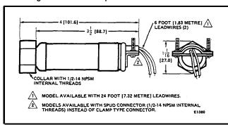
FIG. I- INSTALLATION DIMENSIONS OF THE **C7027A**, IN in. [mm IN BRACKETS].
