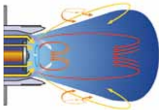
Low NOx emissions: • fuel staging techniques. • two internal air distribution circuits.
