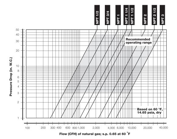
A minimum of 3 in. W.C. Δp is required when sizing at maximum flow capacity for optimal control on high turndown applications (40:1). A 2 in. W.C. Δp can be applied for sizing if a lower turndown (in the range of 10:1) is required. Sizing the FRG/6 using a 1 in. W.C. Δp or less is not recommended for most applications.
