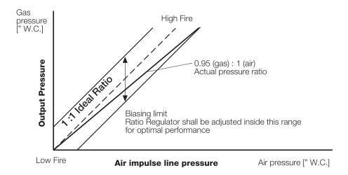
The above illustration shows that the air impulse line can be adjusted to achieve excess air, excess gas, or on ratio at low fire. However, the air impulse line slightly exceeds the gas outlet pressure at high fire rate.
