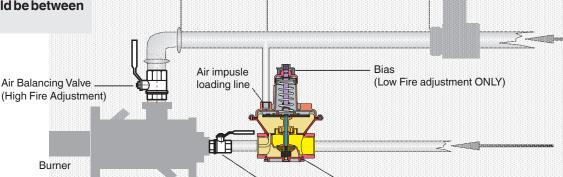
Gas Limiting Valve (High Fire Adjustment)
