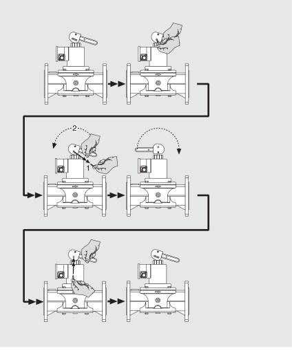
Manually operated safety shut-off valve HSAV HSAV/5
