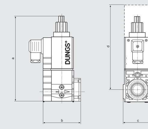
d = Space required for replacing solenoid
