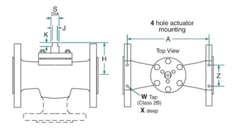
**Actuator mounting dimensions.**Full dimensions for valve and actuator assemblies are available
